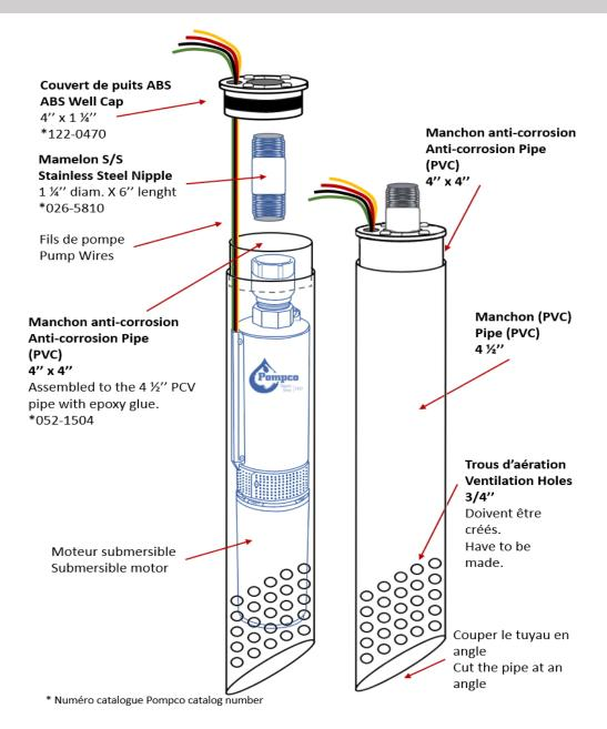
In all cases, the pump must be supported at 15 degree slant to assure proper bearings lubrification whether the pump be placed near the slope or in the bottom. Shield the pump from direct physical contact. Protect and screen the pump intake to prevent blockage by leaves and weeds, but remember the need for an adequate flow over the motor and the entry of the pump. In addition, protect the entire underwater installation from water currents, ice, etc.
